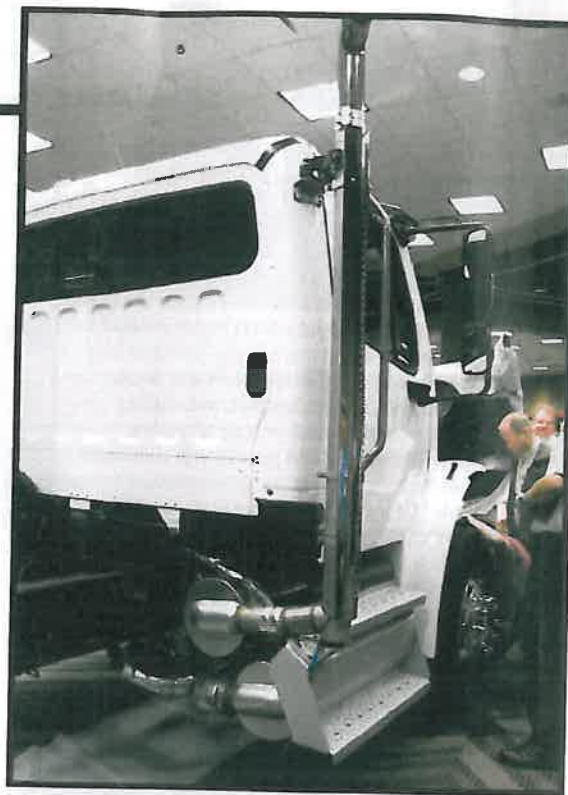
Most SCR components of the exhaust system on this medium-duty Freightliner M2 are under the cab, while the tailpipe runs up the right rear. This leaves the frame clear for easy mounting of big bodies. Freightliner showed more than two dozen configurations to mount the components at the NTEA show.
